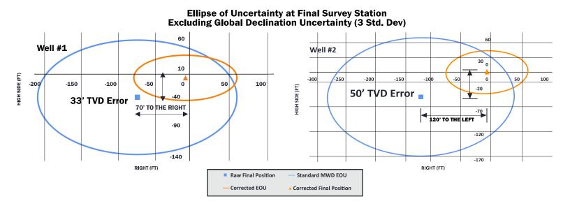
On both Well #1 & Well #2, a build tendency of approximately 1°/100ft combined with pattern downward sliding to combat it were the primary cause of the TVD error identified. HiFi Nav is able to identify and account for the characteristics of the wellbore trajectory that go unnoticed by traditional MWD surveying practices by synthesizing all available drilling data to model the trajectory at 15ft intervals.
